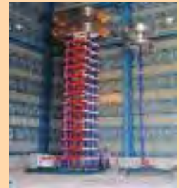
2400kV, 240kJ Impulse Voltage Generator
