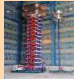
2400kV, 240kJ Impulse Voltage Generator
