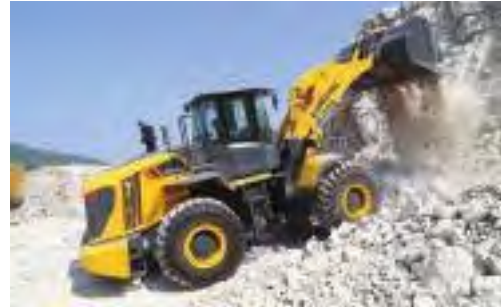
The 856H's new cab design allows for improved visibility to the work tool and improves all-around visibility for safety
