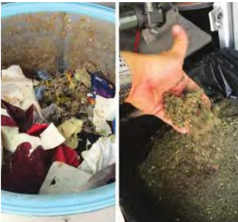
Dry, sterilised, inert processed garbage or RDF resembling 'fluff' is created out of the miscellaneous garbage that may include glass, food, steel, rubber, amongst other waste matter. (Photo: MAC)
