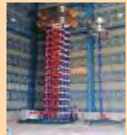
2400kV, 240kJ Impulse Voltage Generator
