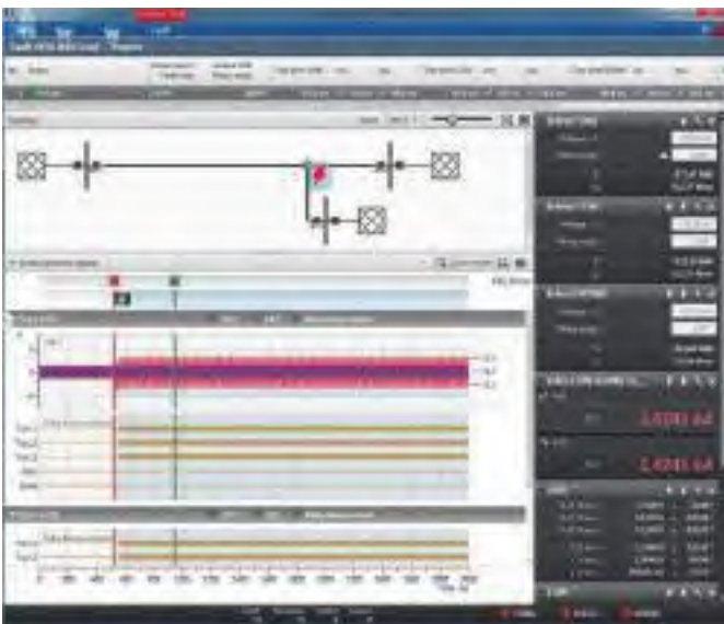
Figure 1: RelaySimTest during testing at Illwerke AG. Even considerably more complex networks are easy to model using the integrated editor.
