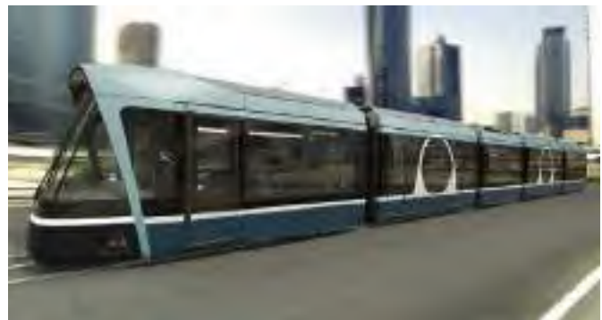
A Citadis tram single unit measures 33 metres in length and can accommodate 207 passengers. (Photo: Alstom)
