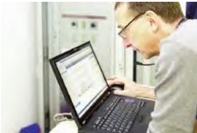
Figure 4: Just one PC is used to control all three protection ends and assess the results.
