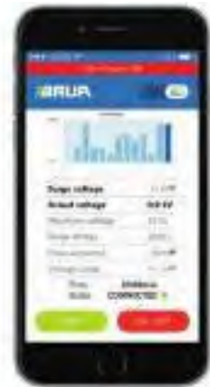
Testing and diagnostic functions of the titron test van can be remotely controlled via a new "Remote App" available for Android and iOS smartphones, which displays fault location and information via BAUR GeoBase Map technology.
