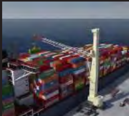
The new variant of its diesel-electric Terex Gottwald Model 8 mobile harbour crane has a loading capacity of more than 8,800 standard containers.
