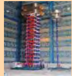
2400kV, 240kJ Impulse Voltage Generator
