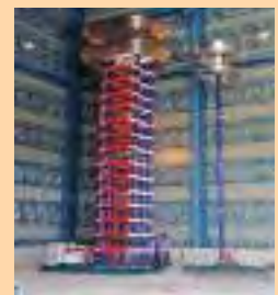
2400kV, 240kJ Impulse Voltage Generator
