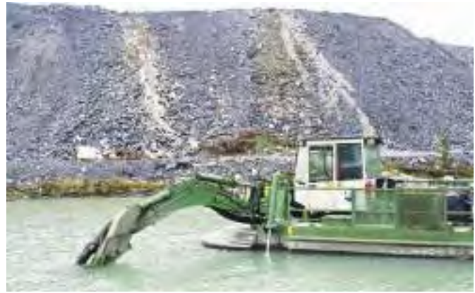
Watermaster dredger pumps sediments from a process water pond at a gold mine. (Photo: Aquamec)
