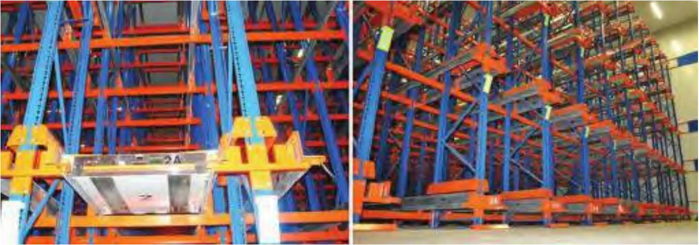
ARCOMA satellite system combines the density of drive-in systems with the benefits of pallet-flow systems and can be easily positioned and repositioned by lift trucks of an existing fleet.
