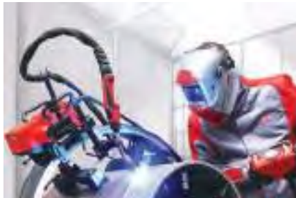
The FlexTrack 45 Pro rail-mounted welding carriage is suitable for use in the construction of containers, power stations, bridges, ships and vehicles.
