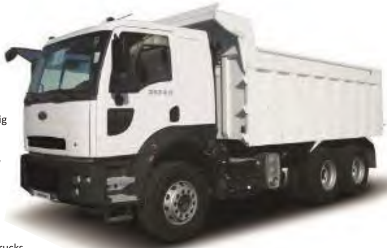
Ford's 2532D truck is from the Hot Climate Package that provides comfort in hot and dusty environments with increased air conditioner performance, improved radiator and filtration.
