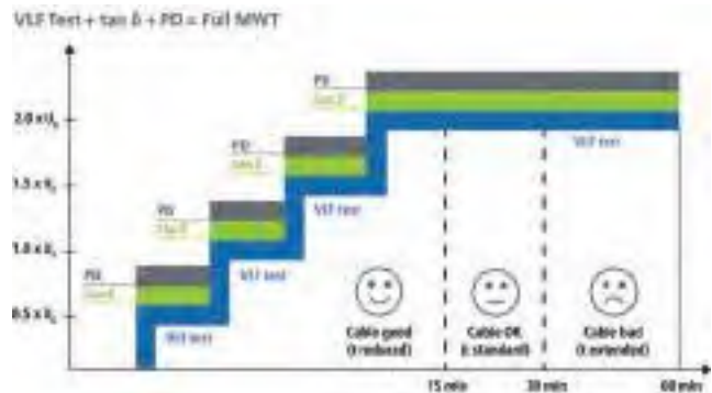
Time-saving combination during the full MWT – the cable testing is completed and the dissipation factor and the PD activities of a cable route are measured in a single flow.
