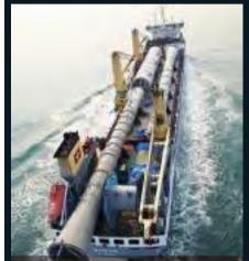
A delivery bound for Saudi Arabia which required Coordinadora's transport designs and on board engineering with force calculated sea fastenings to offset the cargo overhanging the stern of the vessel. operations by highly qualified personnel; and reliability and a well-known reputation in the international market.
