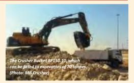
MB crusher uses exclusive and patented Made in Italy technology and is built to process all extracted materials, in order to render it reusable directly onsite. The precision of production aims to allow materials that were previously destined solely for disposal to be processed in calibrated batches, which can be resold or reused onsite, thus leaving the mineral balance of the quarry unaltered.
