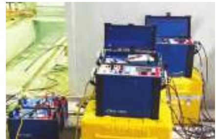
Figure 2: Light-weight and compact HV source with CPC 100 and matching transformers.
