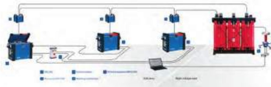
Figure 4: Synchronising up to three CPC 100 to create a HV source with up to 15kVA.
