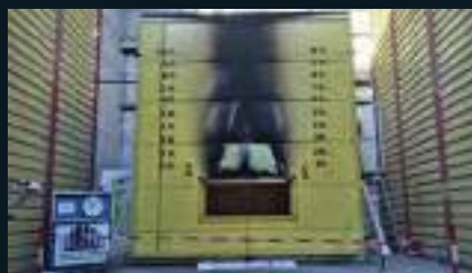
The NFPA 285 tests performed on panels. (Photo: Tiger Profiles)
