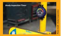
battery is spent. A battery status indicator constantly shows how much power is left.
