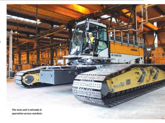
"For barge operation, the available barge load charts for any configuration and any possible counterweight combination are crucial. The modular counterweight system is very good. If a smaller counterweight is sufficient, the unit can also be used on a correspondingly smaller barge.
