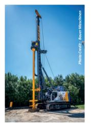
The equipment uses electrical power and operates extremely quietly, making it perfect for use in cities.
