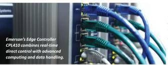
deterministic control in a single compact device. These devices effectively have `two sides of a brain', with the left side being where intelligent sensor data is gathered and real-time deterministic control is provided. Meanwhile, the right side has a software stack running on Linux to deliver the data processing and analytics, dashboards, data logging, and remote monitoring and diagnostics.
