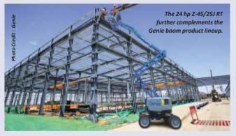
terrain with 45% gradeability, 4WD, traction control, and active oscillating axle. Contributing to ease of service, 90% of the hydraulic hoses are easy to access.
