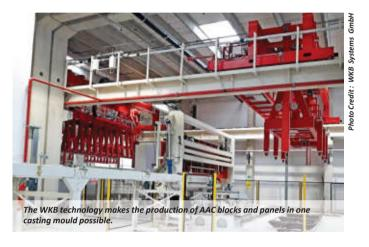
WKB Systems delivered all the equipment needed to make an automated production process possible, including the supply of portal units for automatic insertion and removal of reinforcement frames with cages, dip tanks for anti-corrosive coating and paraffin.
