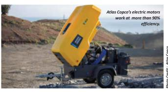
**Maintenance:** Electric compressors have far fewer parts than their diesel alternative, period. This means less to go wrong and maintain. Service intervals are four times longer for diesel compressors – from 500 hours – compared to 2,000 for the E-Air range.
