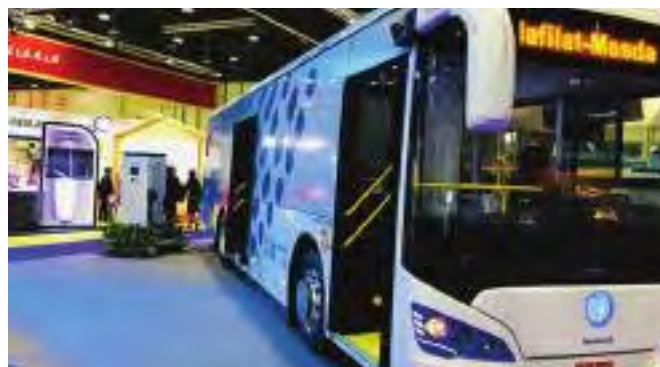
Jointly developed by Masdar, Hafilat Industry LLC and Siemens Middle East, Eco-Bus seats 30 passengers and has a range of 150km per battery charge.
