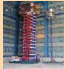
2400kV, 240kJ Impulse Voltage Generator
