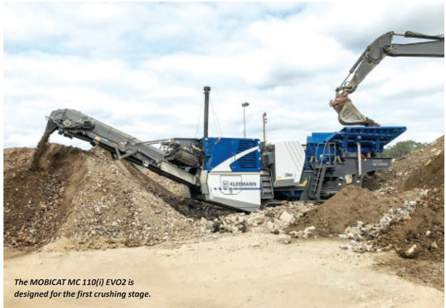
*The MOBICAT MC 110(i) EVO2 is designed for the first crushing stage.*
