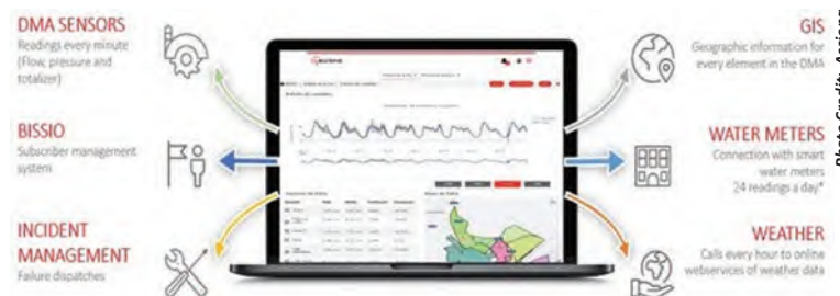
Business Intelligence Of Network Solutions (BIONS) is capable of detecting and predicting problems in water supply networks in real time.
