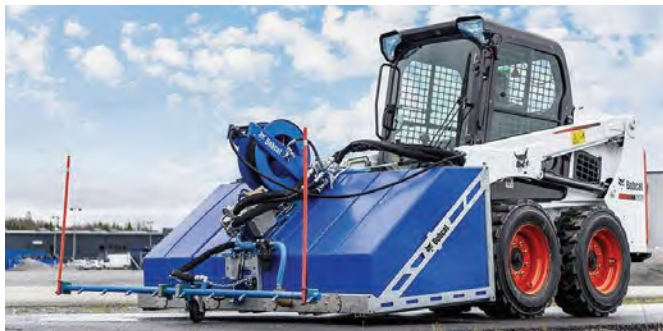
The new attachment is versatile, as the operator can either operate the sprayer from the cab or with a handgun.
