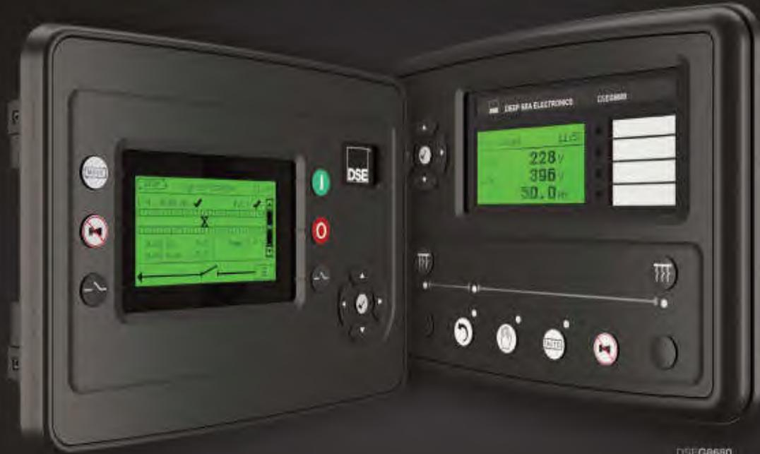
DSEG6600 Parallel Gen-Set Controller with Integral Heater
