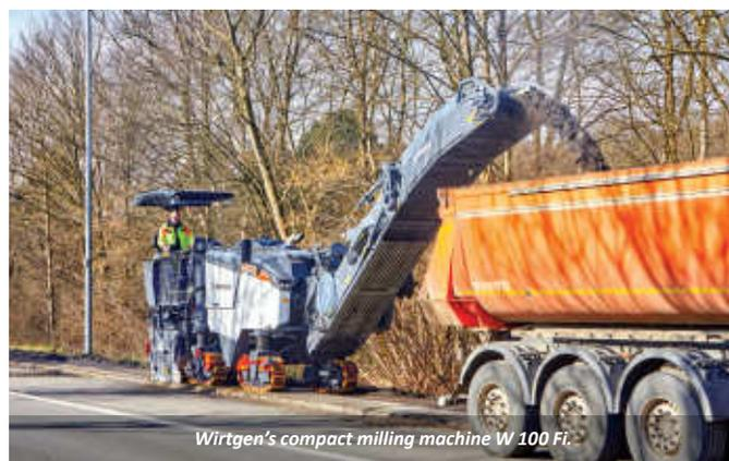
*Wirtgen's compact milling machine W 100 Fi.*
